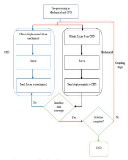
Fig. 1. ANSYS FSI computation process diagram.
