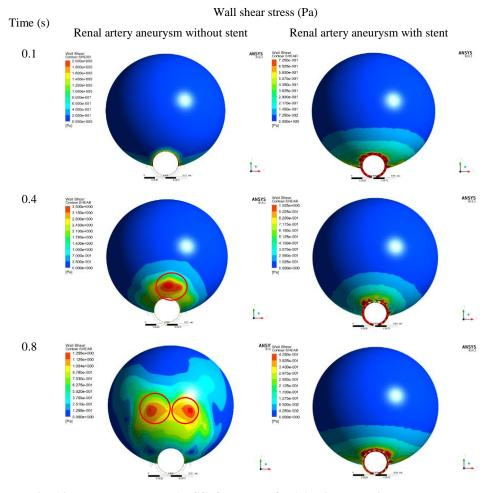
Fig. 10. Wall shear stress (WSS) for cases of RAA with and without stent.
