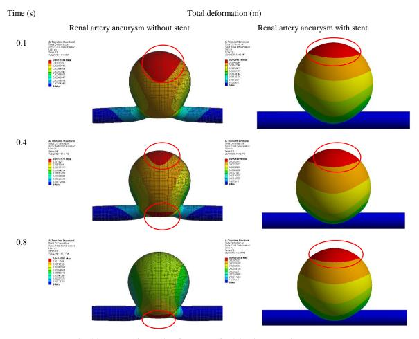
Fig. 11. Total deformation for cases of RAA with and without stent.
