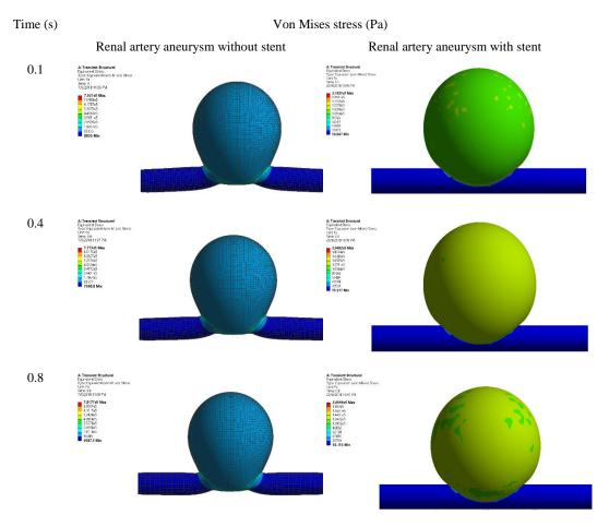
Fig. 12. Von Mises stress for cases of RAA with and without stent.
