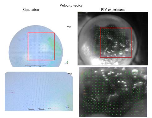
Fig. 8. Velocity vector pattern based on simulation and PIV experiment.
