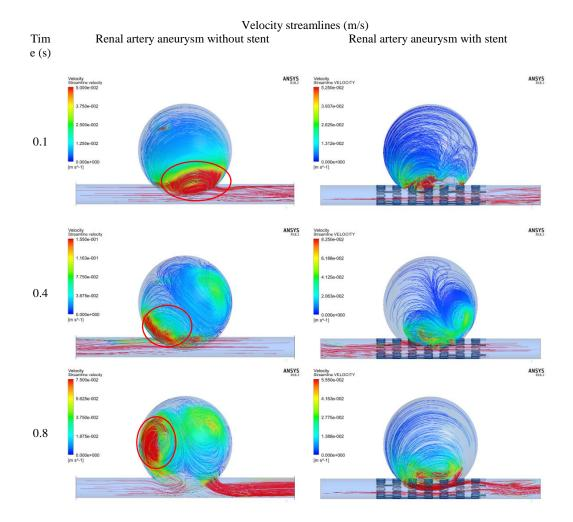
Fig. 9. Velocity streamline for cases of RAA with and without stent.
