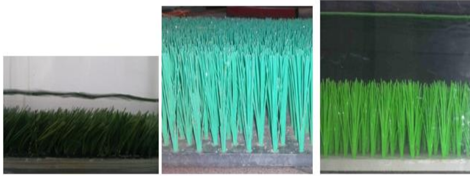
Fig. 1. Picture of the vegetation used for experiments S1 (left), S2 (center) and S3 (right).
