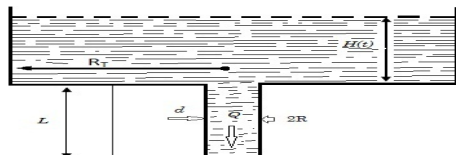
Fig. 1. Tank drainage flow down by mean of circular pipe (Papanastasiou, 1994).
