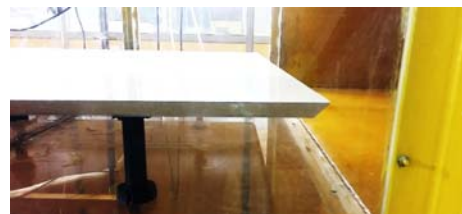
Fig. 7. View of the leading edge of the table which is designed sharply.
