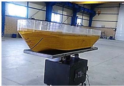
Fig. 6. Measuring moment of inertia using the oscillating table.
