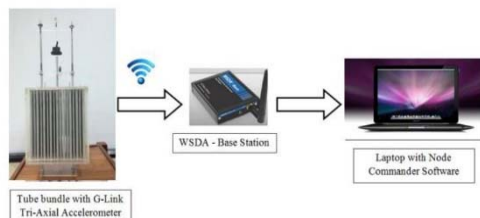
Fig. 3. Data Acquisition System
