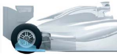
Fig. 1. Diffuser region under a sample car.
