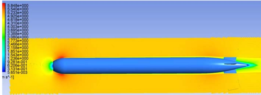
Fig. 4. Contour plot of the velocity field at zero degree of angle of attack.
