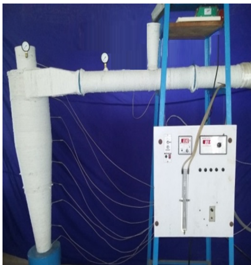
Fig. 7. Experimental setup of cyclone heat exchanger.
