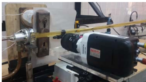
(b) Electromagnetic induction and Camera systems arrangement.
