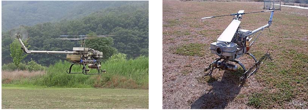
Fig. 1. The agricultural unmanned helicopter for a test bed.
