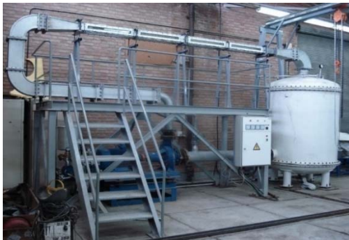
Fig. 1. Closed-circuit water tunnel.
