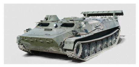
Fig. 1. MT-LB armored carrier in basic version (photo by HSW)
