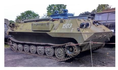
Fig. 14. MT-LBu carrier in the MP-21 command-staff version
