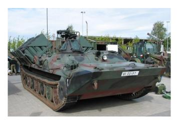
Fig. 6. Scattered mine laying carrier TMN 'Kroton'
