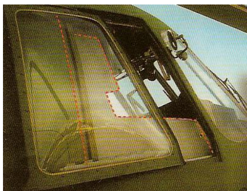
Fig. 10. Mi 8/17 helicopter, the dashed line indicates the position of the armored cover of the pilot's seat Source: [Twaron... n.d.].
