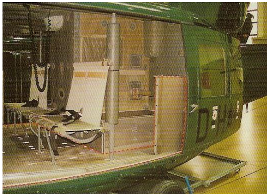
Fig. 9. Design solution for the Bell 212 helicopter against the effects of firing with 7.62 \times 51 AP projectiles. A similar solution was used for Eurocopter NH 90 Source: [Twaron... n.d.].
