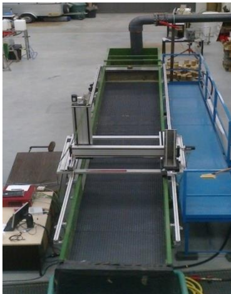
Fig. 1. Open channel flume used in experiments (IMFT, 2015).
