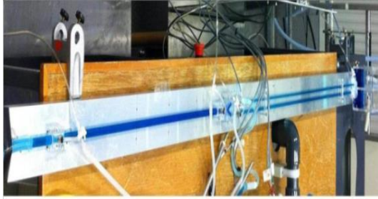
Fig. 2. Experimental setup showing from the left, the header pipe in blue, the Y-splitter, the parallel pipes also in blue and the outlet box.
