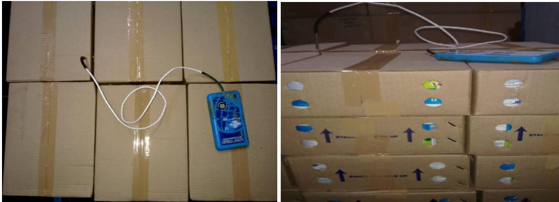
Fig. 5. location of thermocouple at various points in the stack of yogurt
