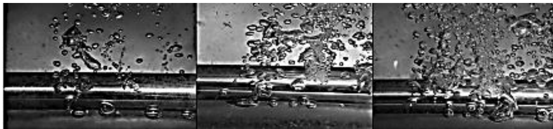
a) Heat flux 15kw/m (b) Heat Flux 40 kw/m 2 (c) Heat flux 90kw/m 2 Fig. 4. Pool boiling of 2-Butanol under the atmospheric pressure
