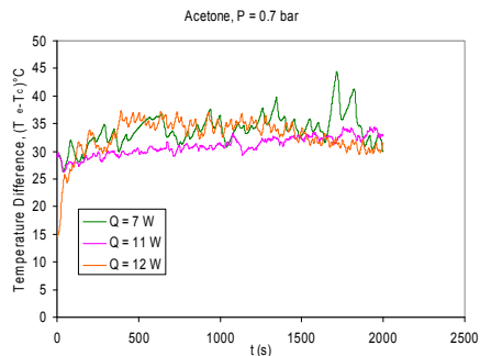
Fig. 4. Effect of heat input on temperature difference for acetone at P = 0.7 bar
