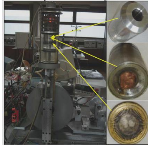
Fig. 3. Photography of the Stirling motor showing the composition of the regenerator
