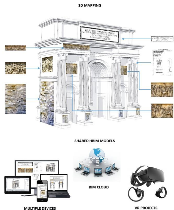
Figure 7. An accurate HBIM model and a proper 3D mapping enabled to achieve the different types of BIM-based analysis, uses, and modern devices, supporting the reading of the model and its mapped information.
