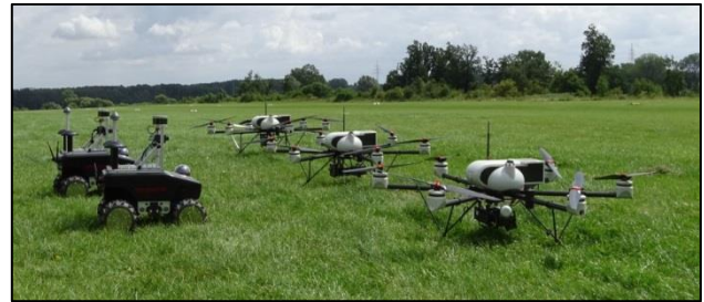
Figure 1: ANKommEn data capturing system, three UAVs Type AR200; and two UGVs Summit XL Robotnik
