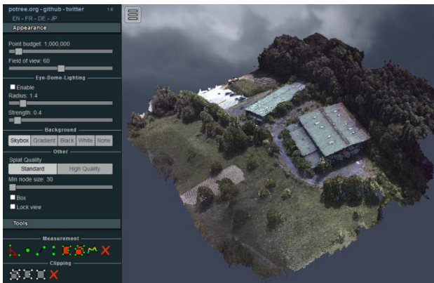
Figure 8: 3D rendering of a large point cloud of the studied area using Potree Converter Tool
