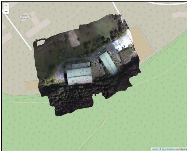
Figure 7: A leaflet based web map created for the orthophoto of the studied area. The orthophoto is published using Geoserver and defined as a layer with its own URL, which is used in leaflet based map.
