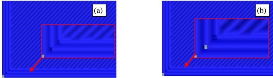
Figure 5. Gap result from slicing process with extrusion width of (a) 0.3 mm, (b) 0.4 mm
