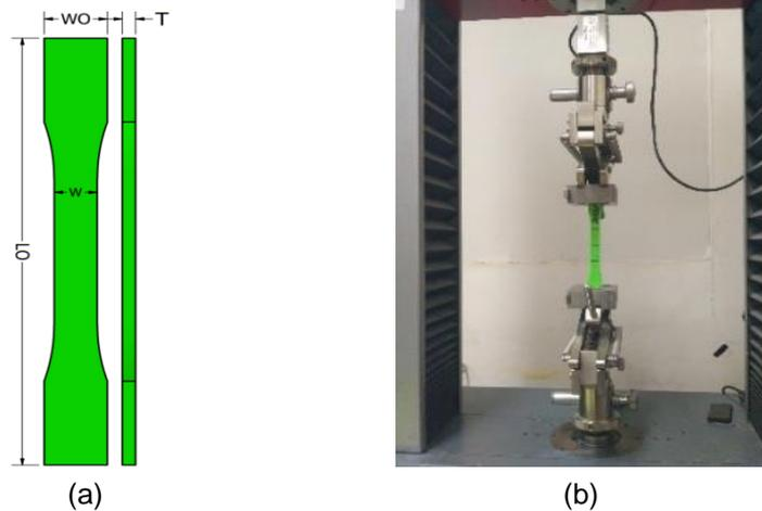
Figure 2. (a) Dimension measurement, (b) Tensile testing
