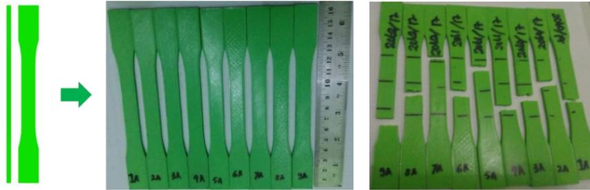
Figure 3. (a) Printed specimens (b) Tested specimens
