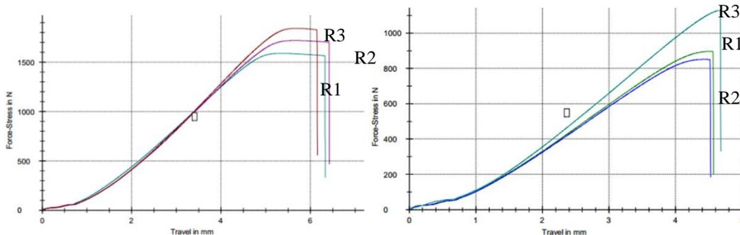
Figure 4. The relation of Load displacement-force of : (a) 5<sup>th</sup> runs , (b) 6<sup>th</sup> runs.
