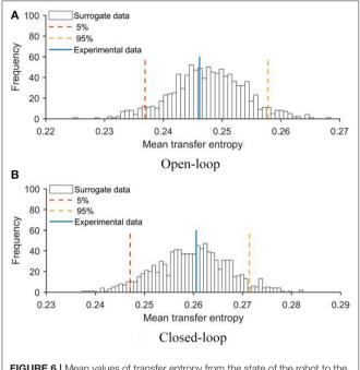
FIGURE 6 | Mean values of transfer entropy from the state of the robot to the horizontal position of the fish compared with surrogate data set for (A) openand (B) closed-loop conditions. Red and yellow lines represent 5 and 95% quantile of the probability distributions, respectively.
