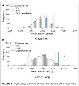
**FIGURE 5** Near values of transfer entropy from the state of the robot to the vertical position of the fish compared with surrogate data set for **(A)** open- and **(B)** closed-loop conditions. Red and yellow lines represent 5 and 95% quantile of the probability distributions, respectively. An asterisk represents a significant (p < 0.050) difference of transfer entropy from chance.
