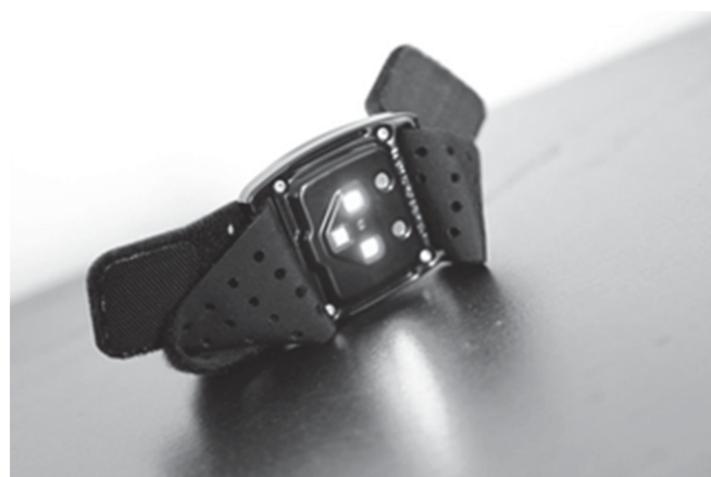
Fig. 1. Example of standard optical sensor for pulse wave registration
