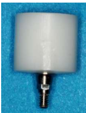
Figure 4: Superstructure cemented to titanium insert
