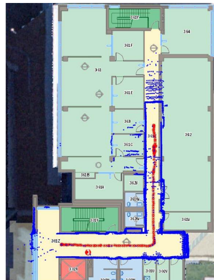
Figure 7. Mapping and position results of the Hector SLAM.
