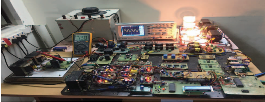
Fig. 19: Photograph for the laboratory setup of MCAEB q-ZSI fed grid system.
