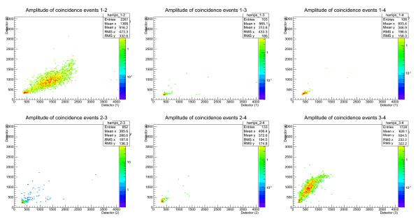
**Fig. 1:** Scatter plot for signal amplitudes in all possible pairs of detectors of the stack. Top left and bottom right plot refer to pairs hosting the <sup>7</sup>Be sample, while the remaining panels show coincidence events for uncorrelated pairs of detectors
