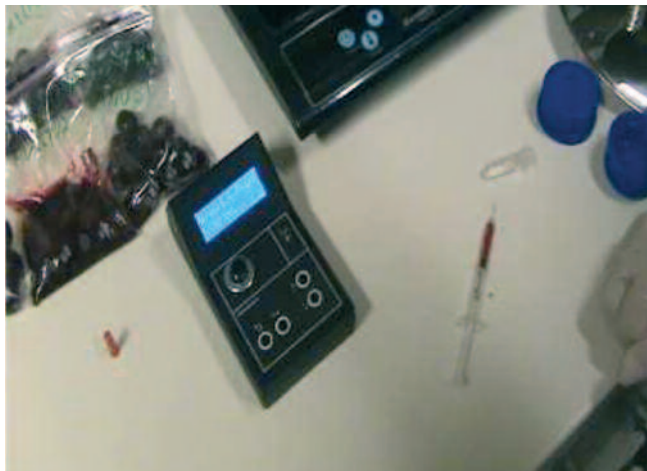
Figure 1. UVEX ML-1, the portable implement and its supplement for the quick measurement of the anthocyanin content of sour cherry fruits
