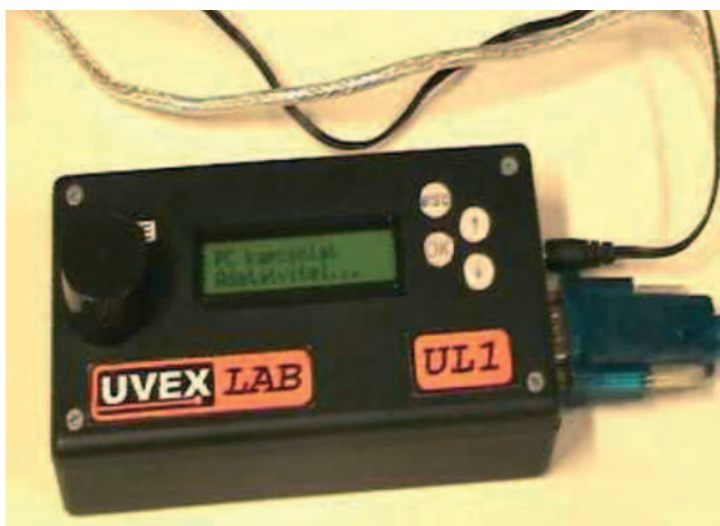
Figure 2. UVEX UL-1, the portable laboratory implement for the quick measurement of the anthocyanin content of sour cherry fruits
