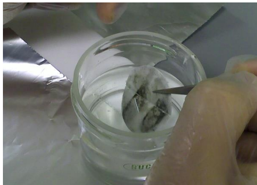
Fig. 5A.- Unfold the filter and introduce it into your container for extraction
