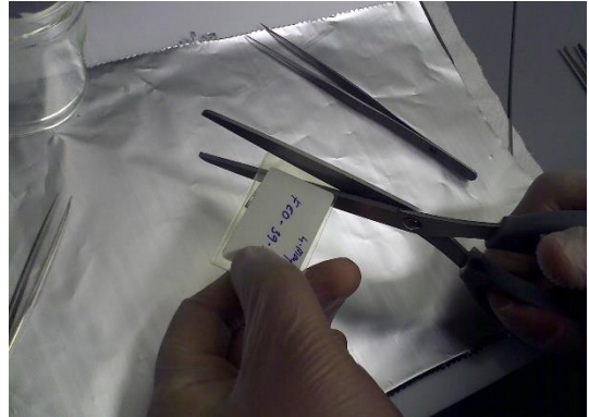
Fig. 2A.- Cut the plastic envelope by the edge
