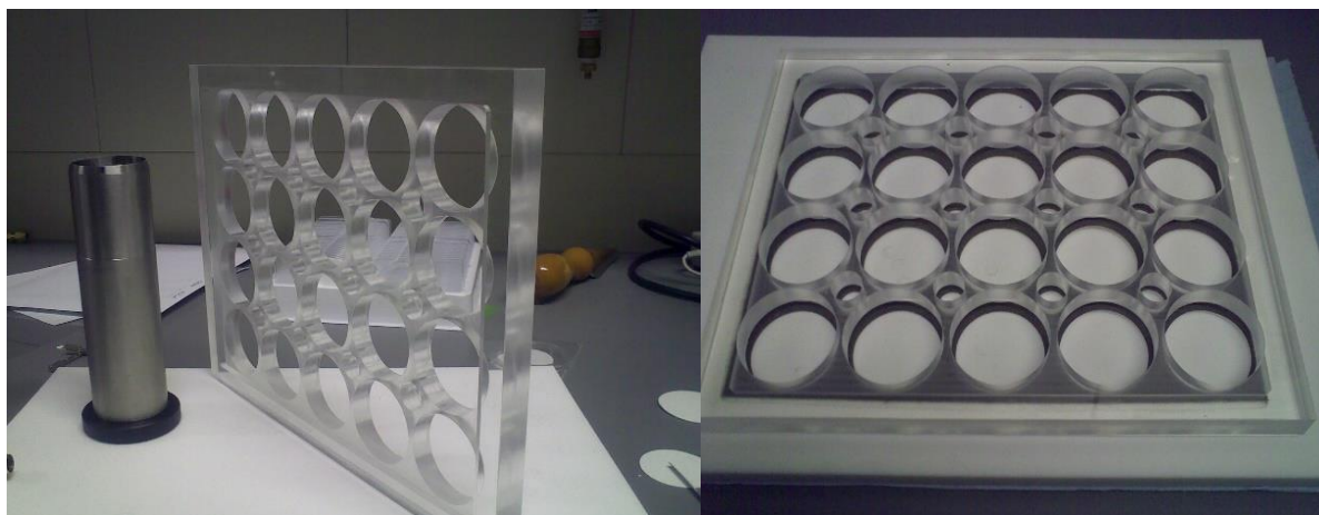
Figure 5 - Mould and tools for the subdivision of the high volume filter
