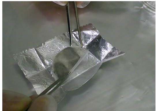
Fig. 4A.- Unwrap the aluminium foil to get the filter
