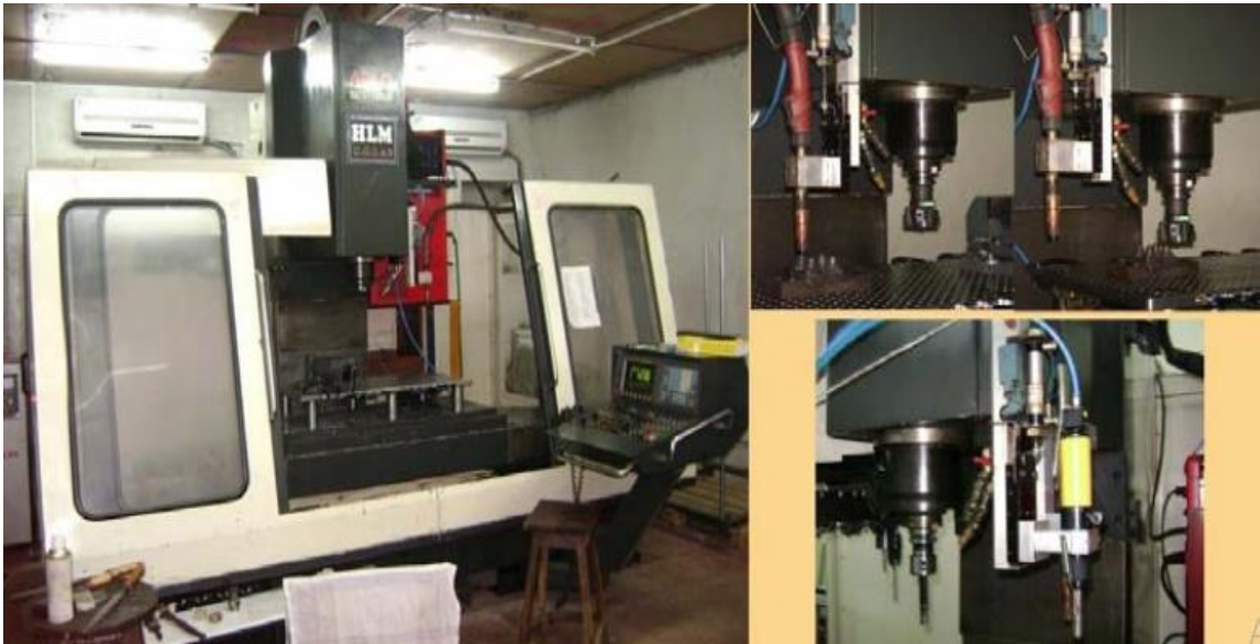
Figure 1.7. A 3-axis ArchHLM machine (integration of Argo 1050P 3- axis CNC machine and Fronius TPS 4000 welding unit) [10]
