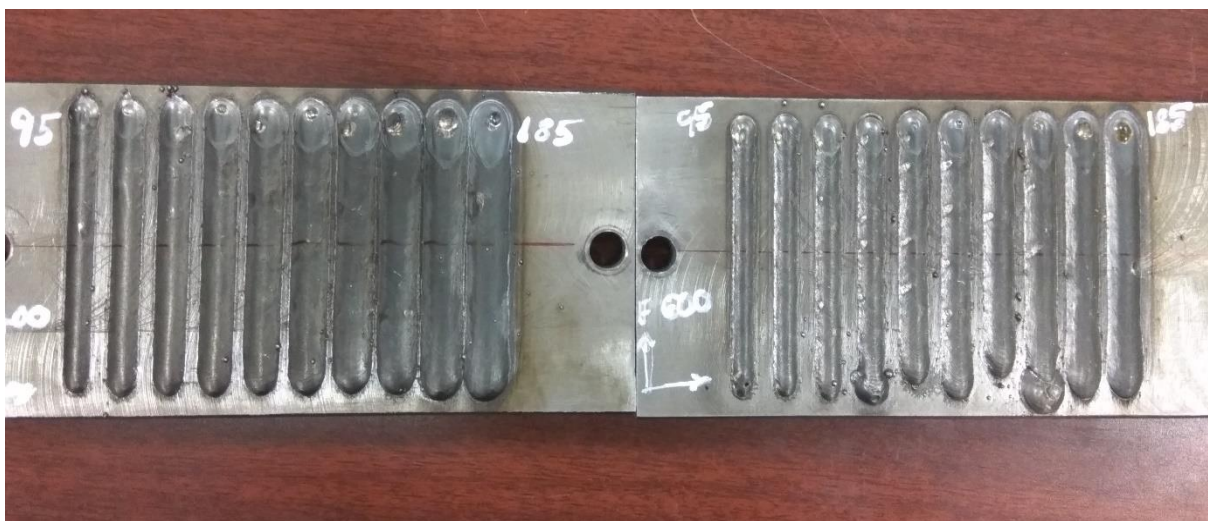
Figure 4.11. Deposited Single bead for torch speed of 400 & 600 mm/min with different current (95-185)
