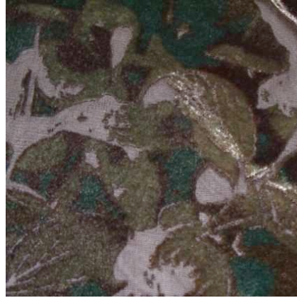
Figure 7: Silk viscose velvet with devore and reactive print on reverse of fabric (21)
