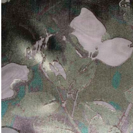
Figure 6: Silk viscose satin with devore and reactive print on reverse of fabric (20)
