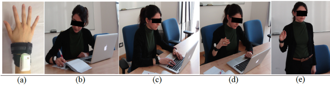
Figure 3.3: (a) The configuration of the EXLs3 sensor on the right hand. (b),(c) The simulated data are collected during daily work activities in the office (e.g., sitting, writing, and typing). (d),(e) The subjects are asked to intermittently perform hand flapping upon receiving a start/stop cue from the instructor.
