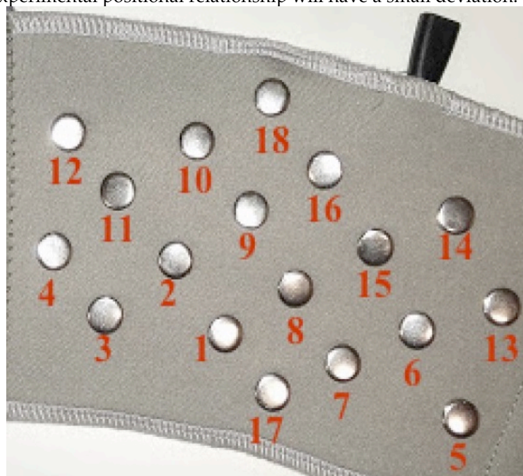
Figure 5. The 2-D arrangement of the experimental electrodes (17 and 18 electrodes are ground wire)
