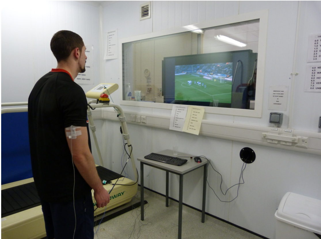
Figure 7. Interior view of the environmental chamber, showing a subject completing an experimental trial.
