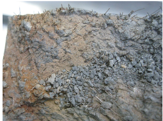
Fig. 12 Fracture surface showing matrix spalling and pulverization
