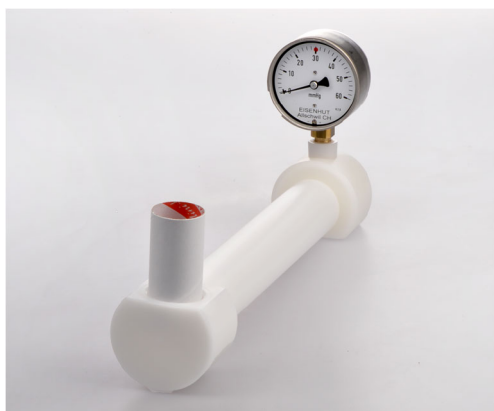
Fig. 2 Figure 2 shows the MR-compatible manometer including the mouth piece, which the volunteer had to hold in his hand during the investigation. Thus, we were able to perform investigations under standardised conditions with target positive pressures of either +10, +20 or +30 mmHg, respectively, or at negative pressures of -10 and -20 mmHg (suction against resistance), respectively
