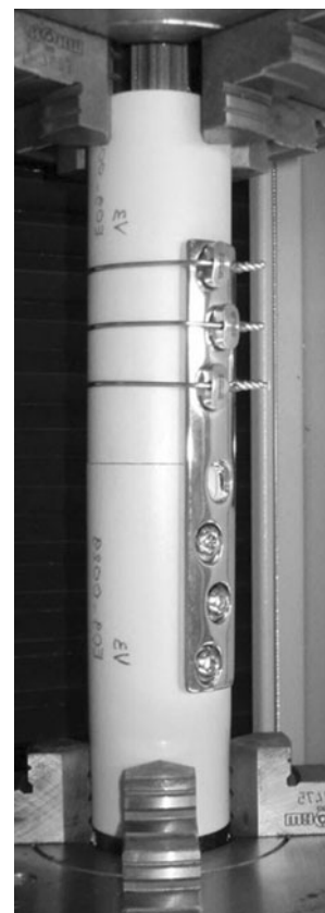
Fig. 4 Photograph of the test setup in the group with the new device in the transverse fracture model in synthetic PUR bone with a revision hip stem in situ. The fracture was fixed using screws distally and the new plate inserts for wire cerclage fixation proximally
