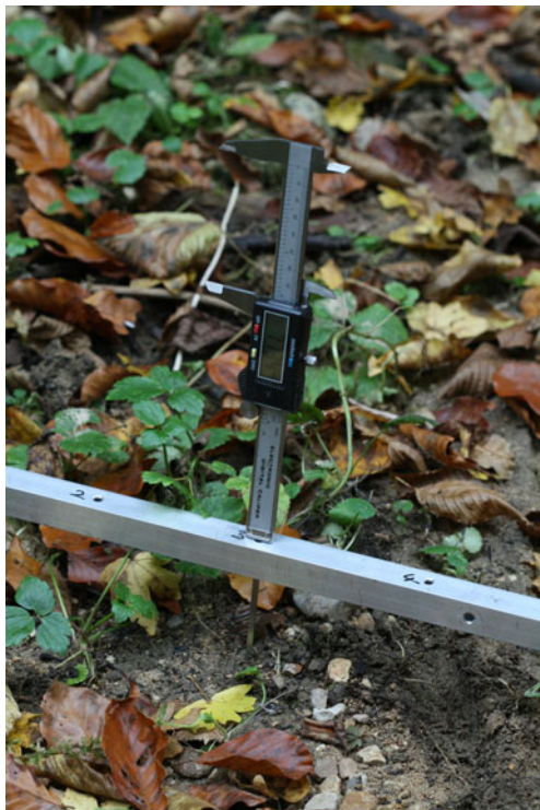
Fig. 4 A digital caliper was systematically mounted onto the profile bridge in order to measure the distance to the underlying soil surface at each of the ten predetermined measurement positions along each transect
