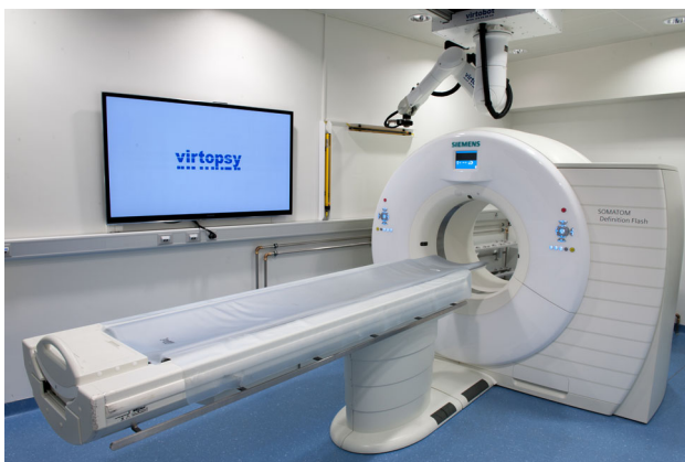
Fig. 2 Virtobot in parking position above the CT gantry. The screen in the background is connected to the computer running the Virtobot software
