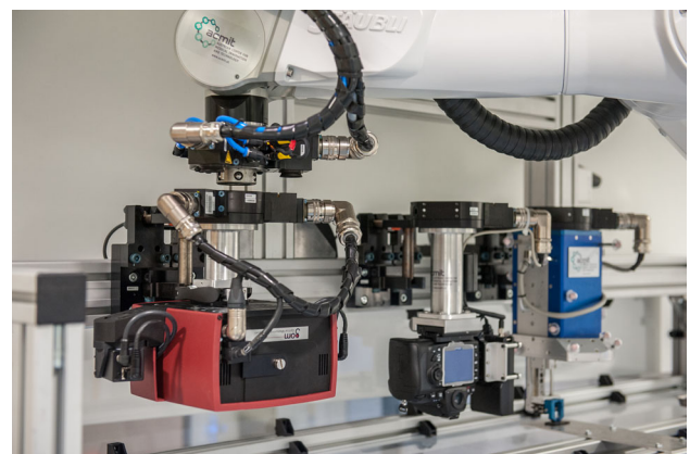
Fig. 3 Tool stand during automatic tool change. Left to right surface scanner, digital photo camera for photogrammetry and biopsy module
