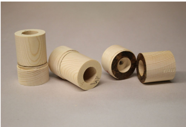
Fig. 3 Cylindrical specimens for interface characterisation of friction welded timber (inner radius R_i = 10 mm, outer radius R_o = 38 mm, wall thickness t = 9 mm, height h = 90 mm)
