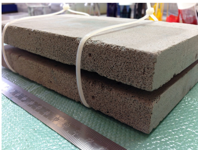
Fig. 2 Ceramic foam plates bound together by standard plastic cable ties
