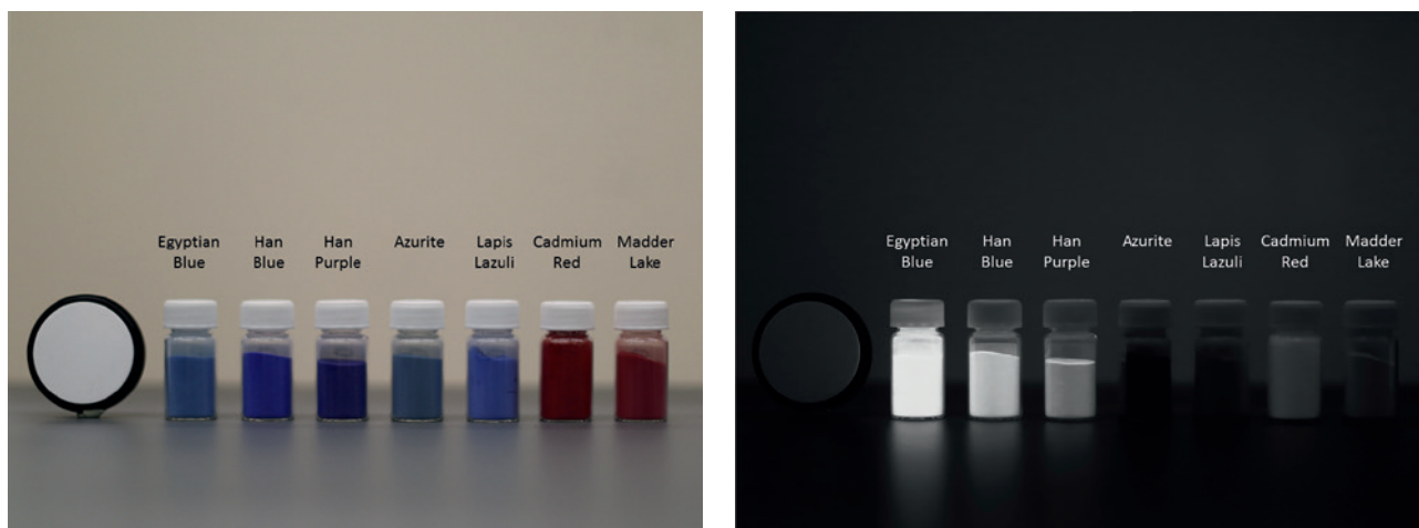
Fig. A2: Visible light photograph and visible-induced infrared luminescence image of several pigments
