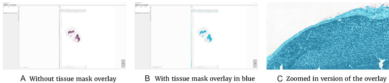
Figure 4: Interface of the ASAP viewer interface. Visible items are the annotations tools in toolbar, the viewport showing the WSI, and the plugin panel on the left.
