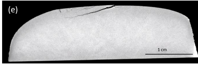
Figure 7: X-ray tomography of the crack network from one of the specimens visualized by 2D slices at different locations within 10 mm along the running direction.
