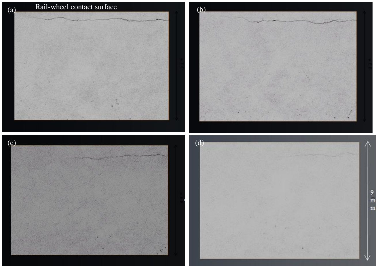
Figure 4: 2D slices showing the crack network within the wing rail at different locations along the longitudinal direction (a) at the transverse cut (0 mm), (b) 10 mm from the transverse cut, (c) 18 mm from the transverse cut and (d) 29 mm from transverse cut.
