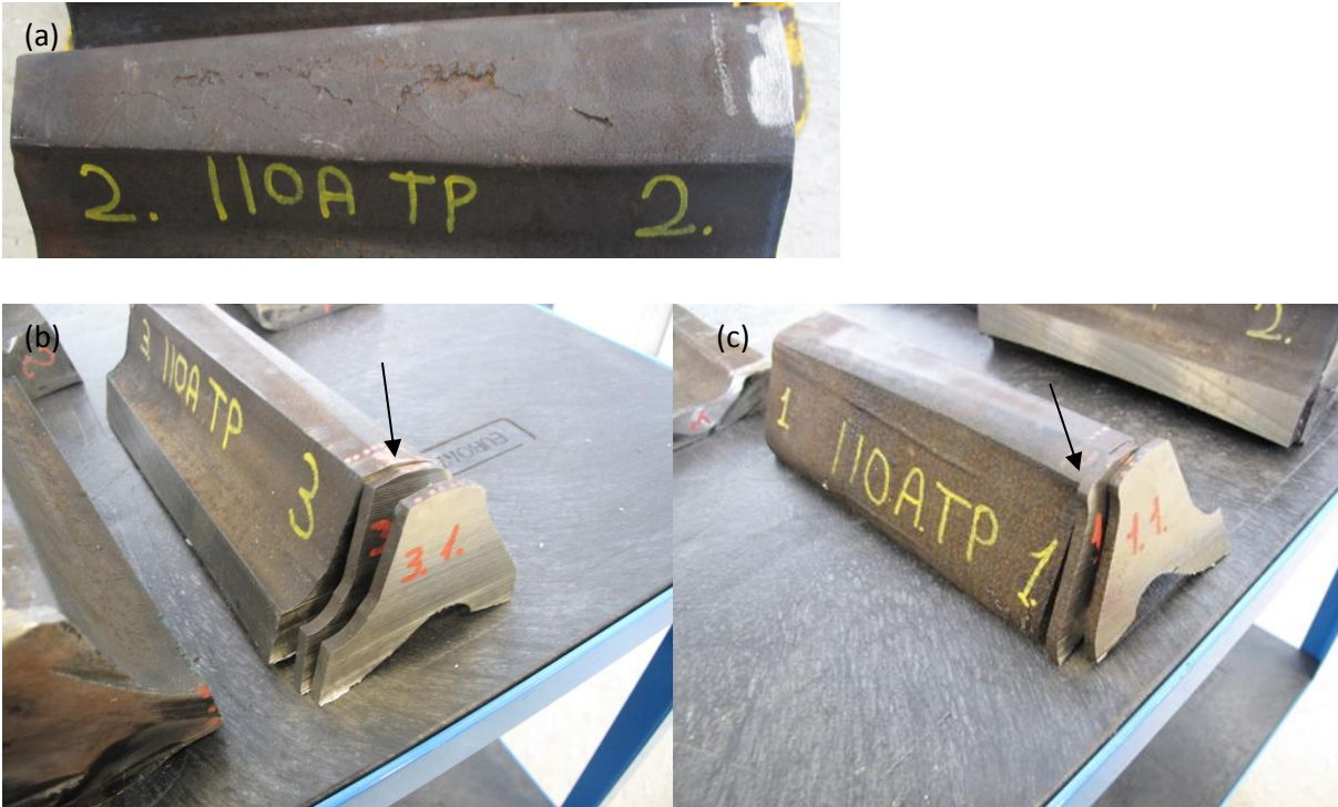
Figure 2.5: Individual components of the ATP 110 crossing after separating them (a) the nose of the crossing showing distinct visual cracking and spallation, (b) and (c) the two wing rails, the rail wheel contact area is evident from the deformation and is marked by arrows.
