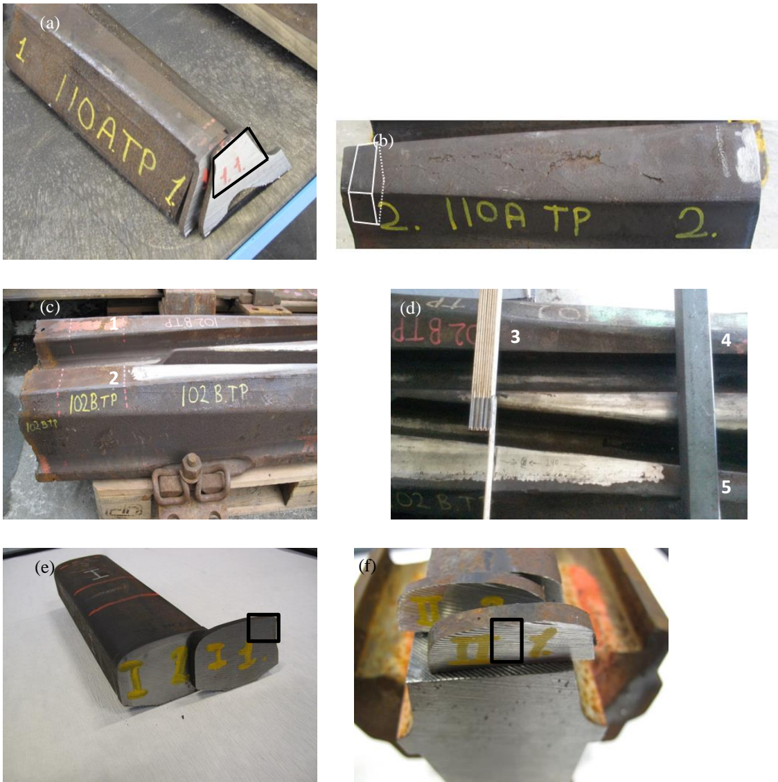
Figure 2.12: The areas where hardness measurements were made on the different components of the crossings (a) ATP 110 manganese wing rail, (b) ATP 110 manganese nose, (c) and (d) BTP 102 manganese crossing, the numbers in the figure indicate the area for hardness profile maps, (e) pearlite wing rail showing the surface of hardness measurements and (f) pearlite nose rail showing the surface of hardness measurement.
