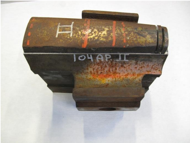
Figure 2.3: The nose of the pearlitic crossing after unbolting and separating it from the crossing showing the pieces cut out for metallurgical investigation.
