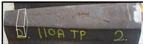
Figure 2.17: Nose of ATP 110 manganese crossing showing the region where specimen for EBSD scanning was obtained.
