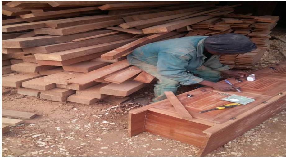
Figure 5.20 A photograph showing work without proper seating and workstation and poor storage of wood depicting lack of sitting stools and inadequate storage space
