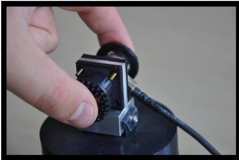
Figure 1. The handle containing the Nano17 force transducer which participants used to lift the experimental objects.
