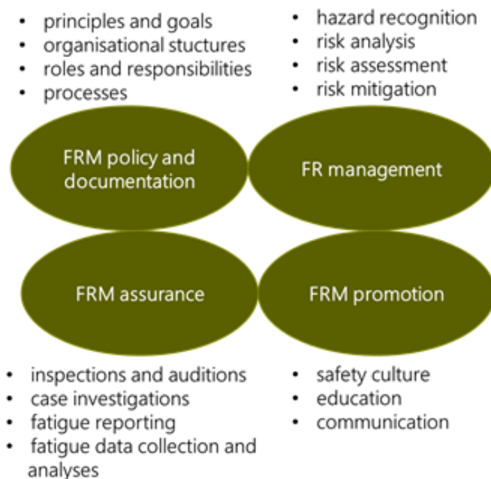
Figure 5.6.1. Four pillar model of Fatigue Risk Management System.
