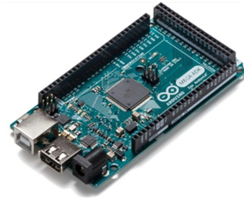
Figure 28. Arduino Mega platform: the selected off-the-shelf microcontroller for the control of the ultrafiltration process of the WUF
