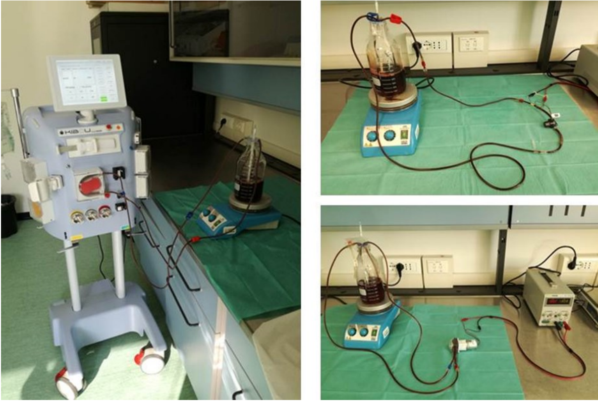
Figure 38. Set up of the in vitro experiment for the three pumps (benchmark pump, centrifugal pump and peristaltic pump).
