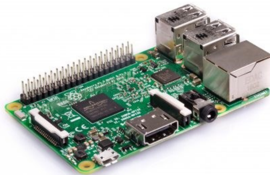
Figure 29. Raspberry PI 3 model B platform: the selected off-the-shelf microcomputer for the management of GUI and data logging of the WUF
