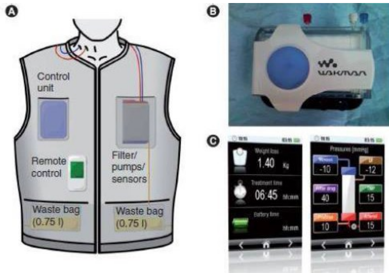
Figure 13. A) . Schematic representation of the WAKMAN; B) Intergrated unit pump-hemofilter; C) Remote control display
