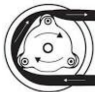
Figure 36. Schematic example of a peristaltic pump
