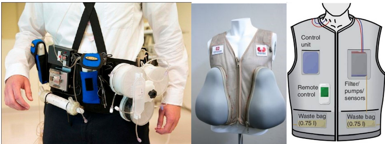
Figure 62. Layout proposal for the WUF: belt-like and jacket.
