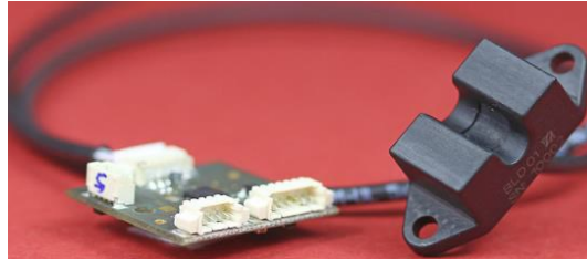
Figure 26. Selected blood leak detector sensor for the WUF
