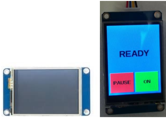
Figure 30. Selected LCD monitor for the WUF
